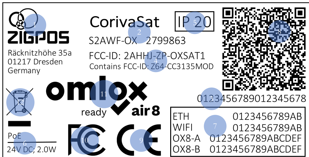
Figure 7 – Example of the CorivaSat nameplate
